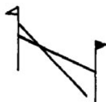
Top end of sloping pole higher than horizontal pole
