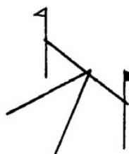
Neither end of sloping poles is supported by standard cup or fitting
