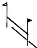
Pole on ground forming false ground line
